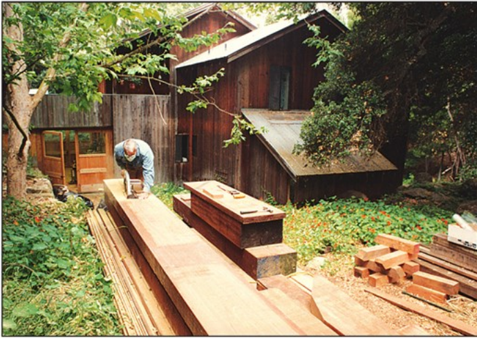
Ken fashioned the yacht's backbone structure from two substantial pieces of balau—a dense, durable, edge-tool-blunting hardwood from the Asia Pacific region.
