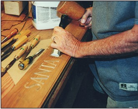
Above —Sometime around 2003, the boat received the name MORNING SONG, and this, and the hailing port, were carved into transom planks. Right —MORNING SONG is planked in 1¼" mahogany. Ken worked alone on this phase of the project.
