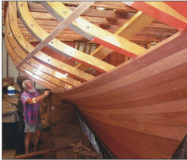
Above —Sometime around 2003, the boat received the name MORNING SONG, and this, and the hailing port, were carved into transom planks. Right —MORNING SONG is planked in 1¼" mahogany. Ken worked alone on this phase of the project.
